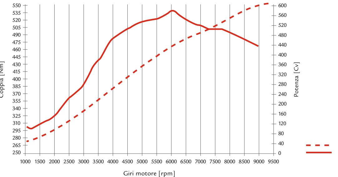
The other main challenge aside from boosting power was to improve torque across the entire power curve. This involved increasing the compression ratio to an exceptional 14:1, the highest value ever achieved by a naturally-aspirated V8, which was achieved by modifying piston geometries.
