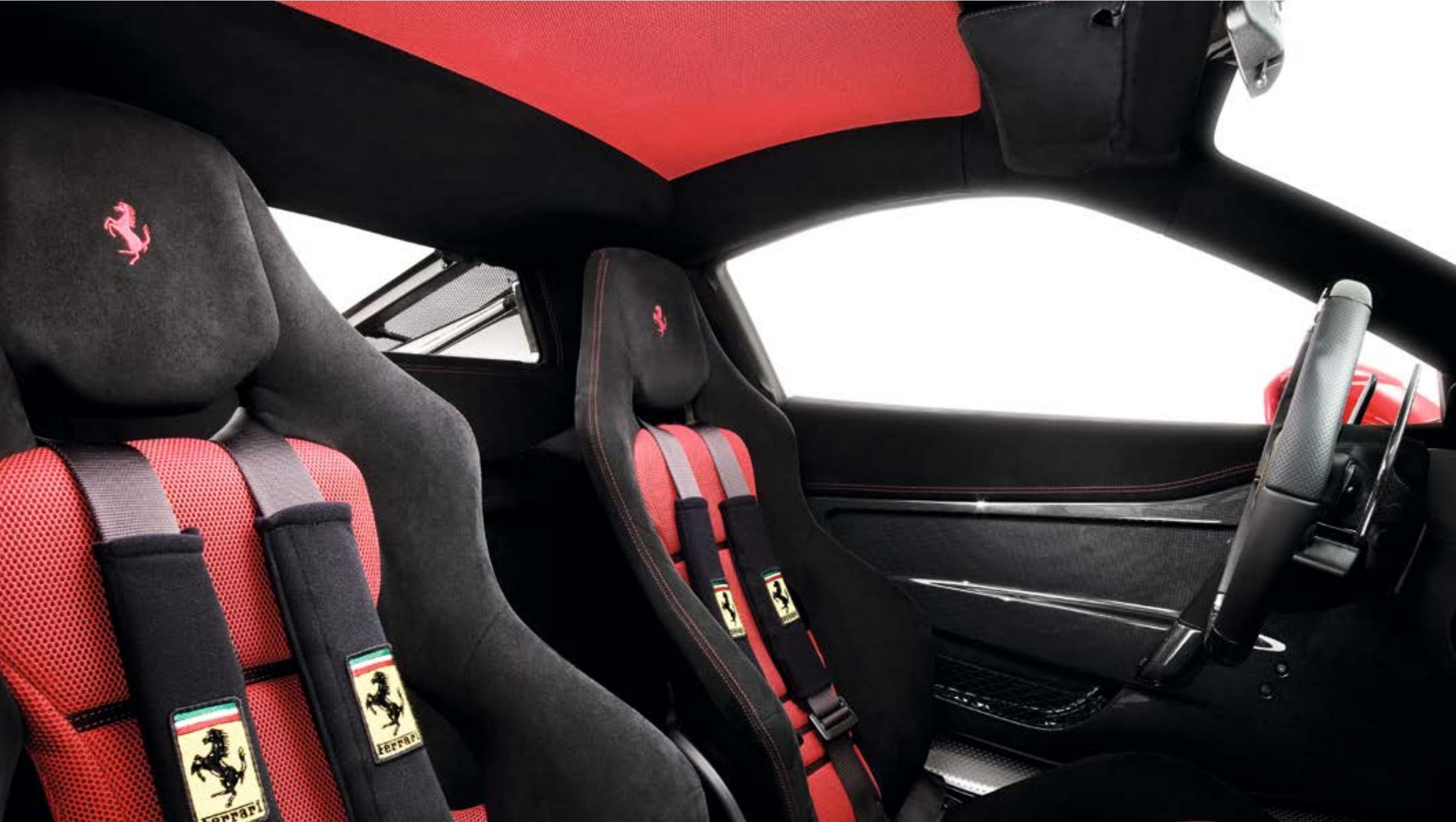
The Sabelt seats have carbon-fibre shells and boast excellent side bolstering thanks to an ergonomic design which also helps contain weight. The shoulder-rests are trimmed in Alcantara for improved grip while seated and the backrests are padded with a breathable 3D fabric to guarantee excellent air circulation and comfort. The same anthracite Alcantara trim with contrasting red stitching also adorns the dash, the door panels, interior and posts.
