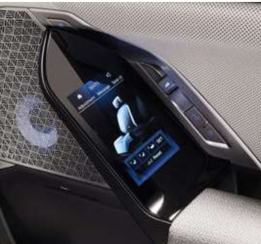
The BMW Touch Command are built-in touch screens in the door panels. Touch Command also allows passengers to operate the radio, paired smartphone, My Modes, rear seat adjustments, roller blinds, climate control and lighting.
