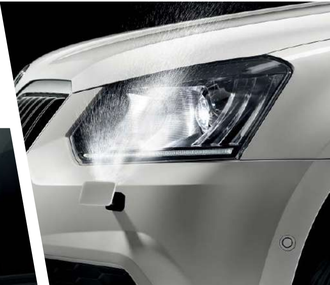
The integrated telescopic headlamp washers keep the headlamps perfectly clean.
