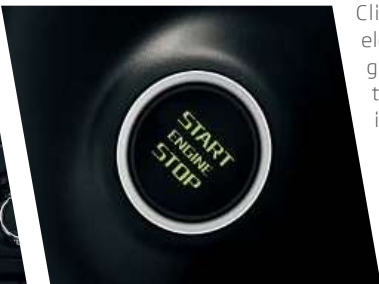
The KESSY system (Keyless Entry, Start and exit System) enables you to use the car without a key. To switch the engine on and off you simply use the Start/Stop button.
