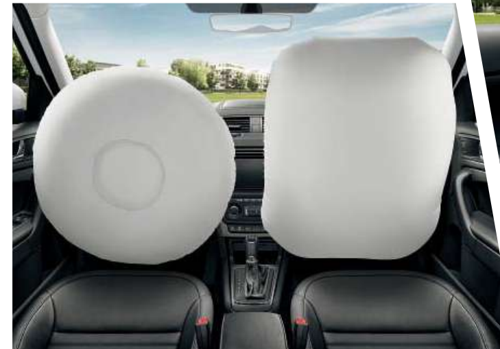
While the driver airbag is hidden in the steering wheel, the passenger airbag is located in the dashboard. If needed, it can be deactivated so that you can fit a child seat in the front seat.
