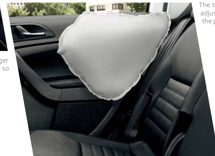
The front and rear side airbags protect the pelvis and chest of the driver and other passengers in the event of a side collision.
