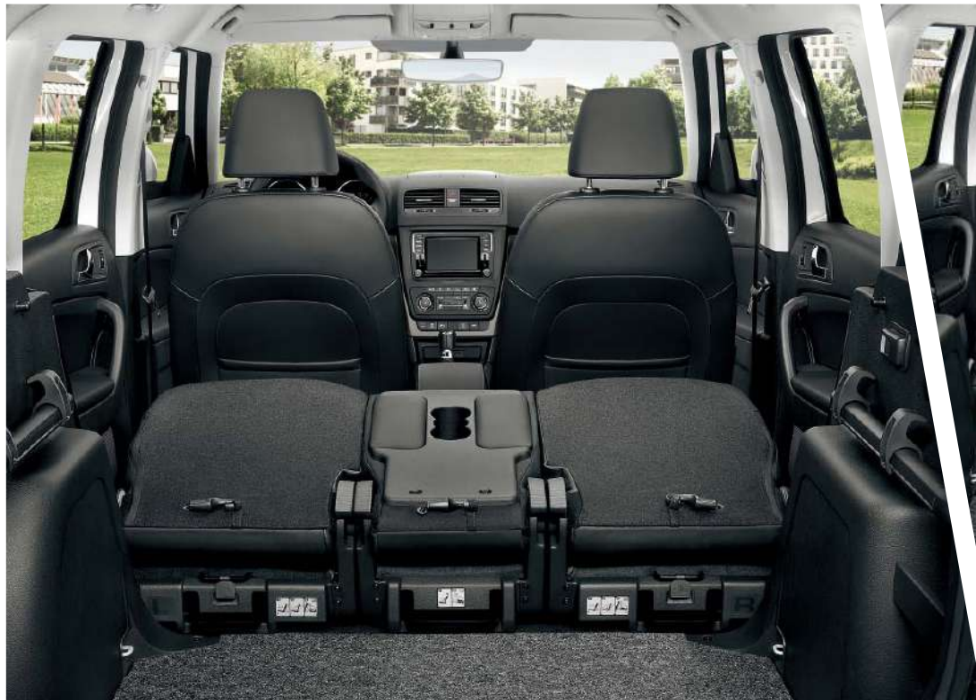
The backrests of the rear seats may be completely folded down towards the sitting sections.
