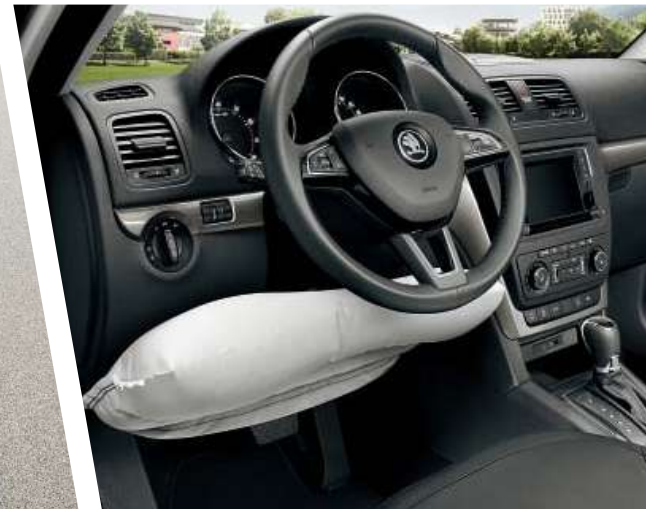
The driver knee airbag prevents contact with the lower part of the dashboard in the event of a collision.
