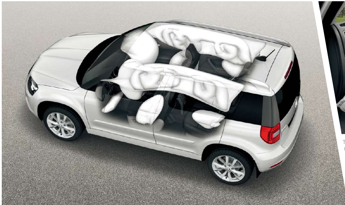
The head airbags, which create a "wall" along the side windows when activated, protect passengers' heads in the front and rear.
